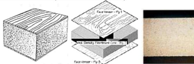
is defined a product that is much in the same manner as particleboard using the latest in manufacturing technology and consists of recycled wood particles that are softened in steam vats called digesters. The softened particles are refined to individual fibers, dried, mixed with resin, and formed into mats. The mats enter a heated press and are cured, becoming panels. Panels are then typically sanded, graded and cut to the appropriate size.
