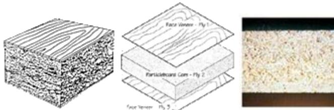
is defined as a wood panel made from recycled wood particles which are not softened and refined. The wood particles are milled to sizes appropriate for the face or core of the panels before introducing the resin and forming into mats.
