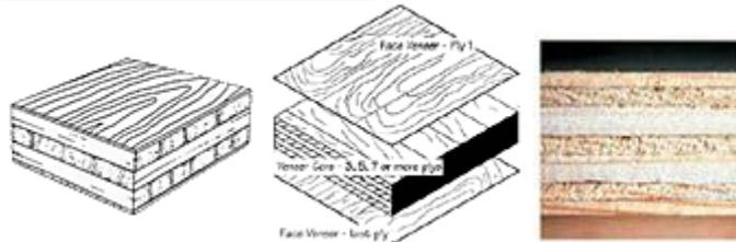
is defined as plywood which all the plies are made of veneer . The directions of the grain in adjacent plies are normally at right angles, with the outer and inner plies placed symmetrically on each side of a middle ply or core. Adhesive is applied to the veneer and pressed together.
