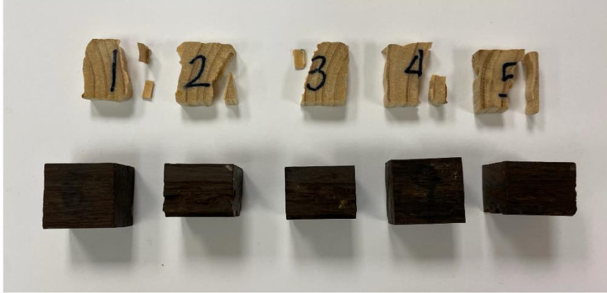
Figure 1. All samples at 28 days of testing against Formosan subterranean termites.
